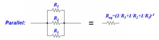
Adding resistors in series and parallel follows very simple rules that should make sense to us. Resistors in series just add to make a larger resistance.  $R = R_1 + R_2 + R_3 + ...$  while resistors in
