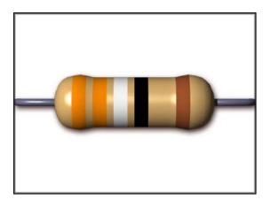
The colored stripes tell us what the value is of the resistor. Only the first three stripes are used for this purpose. The first two stripes are read like a regular number with each color representing a specific digit.
